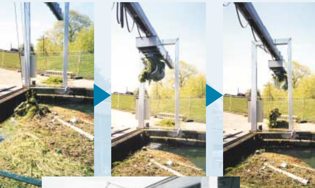
A Bosker overhead gantry machine operating fully automatically under very heavy debris conditions.
